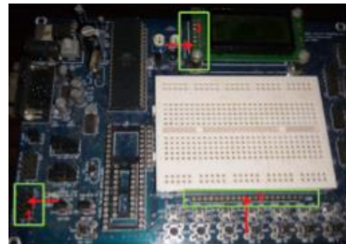
Gambar 1b. Pin header Port IC Atmega8535
